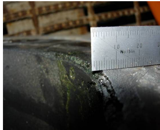
TomoView S-,A-,&C-scan display showing erosion on raised face & actual inspected flange image
