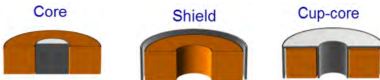
Figure 5.6 Coil with some core material, and types of coil shielding
