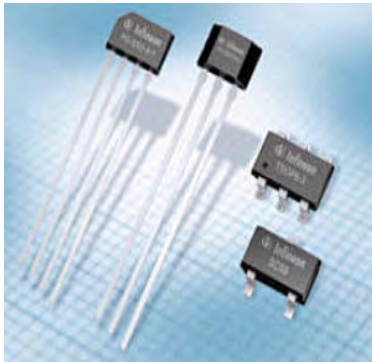
Figure 5.2 Hall effect sensors are usually just IC's
