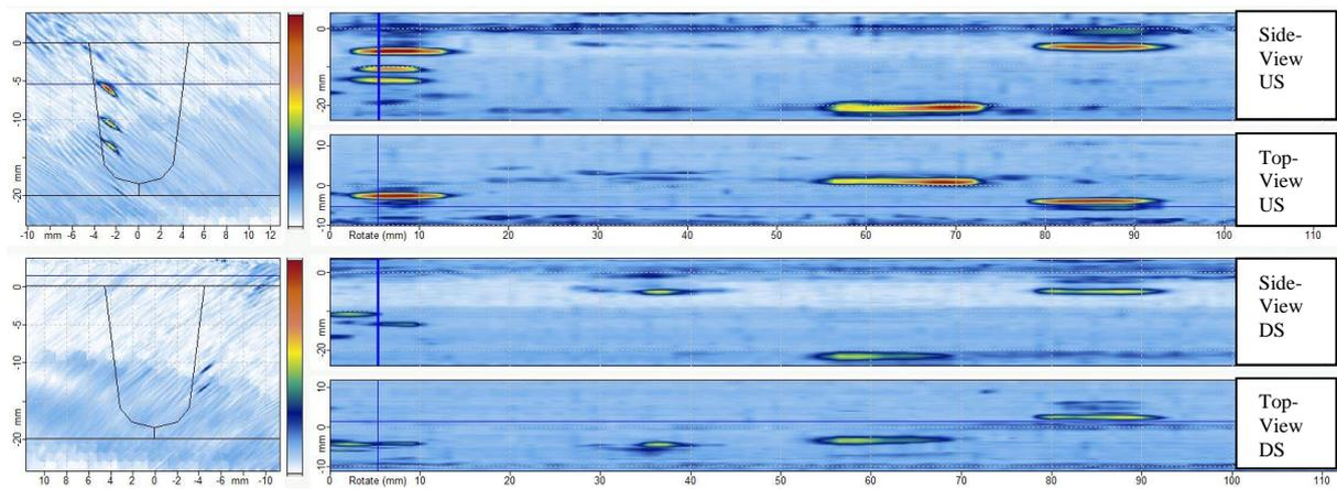
**Figure 9** TFM view of weld examination
